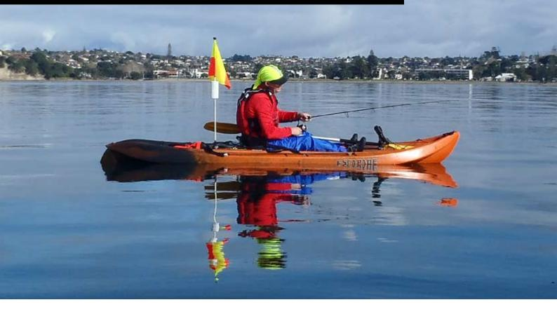
From the manufacturer: The Escapade is a multipurpose kayak suitable for touring and fun in the waves. The Escapade has an innovative 'tri-keeled' hull to give greater speed and stability, especially when loaded with skuba diving equipment or fishing gear. The hull shape and upswept bow ensure good surfing in the waves.
